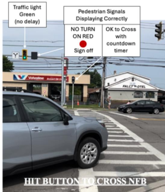
Figure 2. When pedestrian indicate the desire to cross NFB the OK to cross signal illuminates at the same time that the green light for cars turns on.
